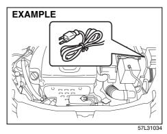
The engine block heater will help you start the engine more easily in very cold weather  $(-18^{\circ}C (0^{\circ}F) \text{ or below})$ . To use the engine block heater:
